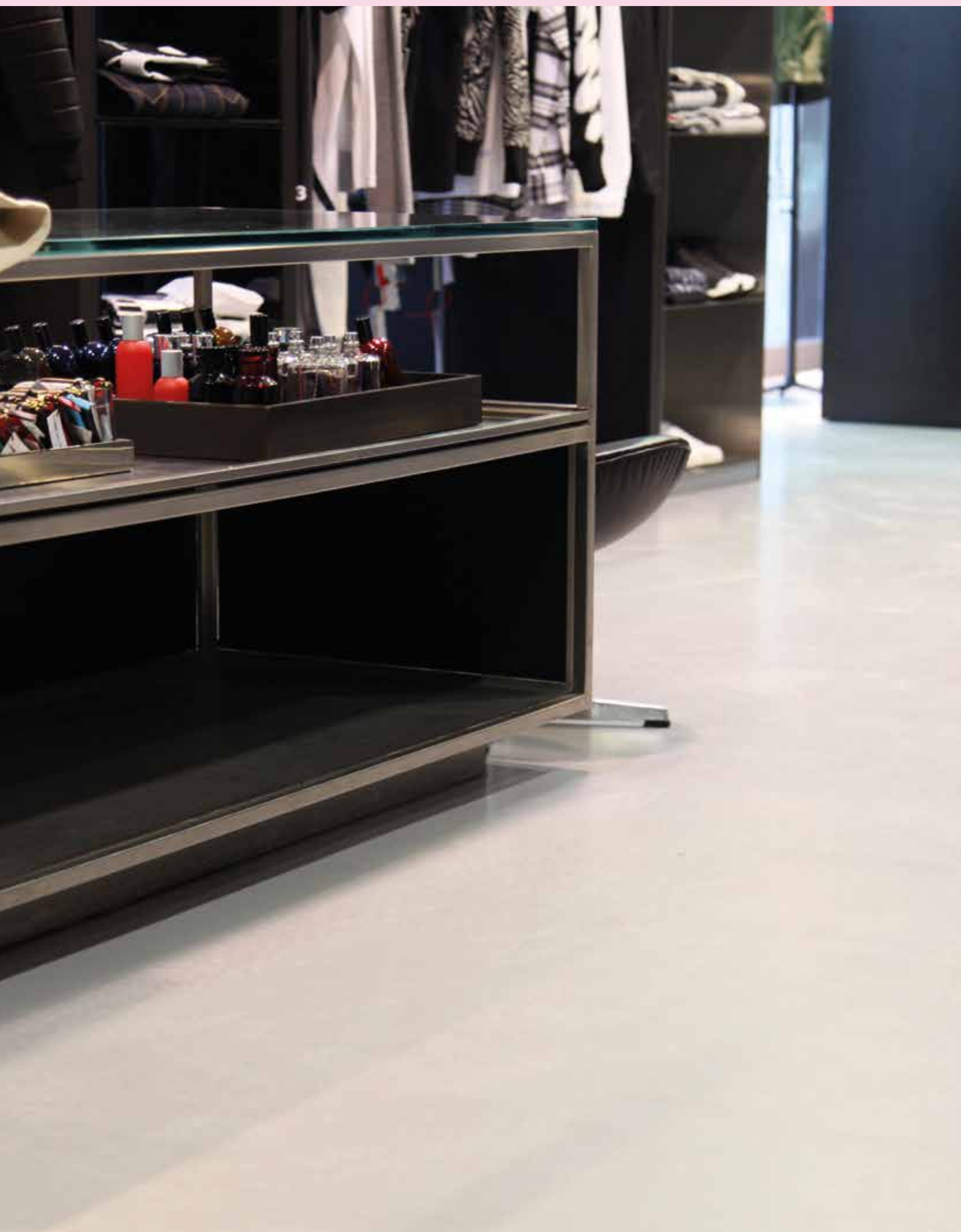
JULIAN FASHION - Milano Marittima, Ravenna, Italy Coating of existing flooring with DRACOFLOOR MD integrated resin system (satin finish).
