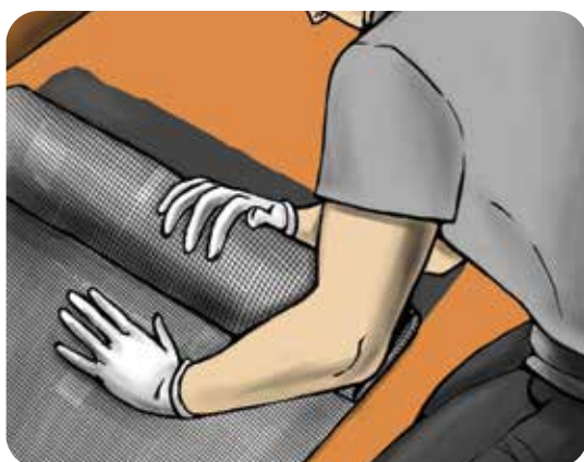
• Lay MAGINET over the first coat of MAGIFLEX while it is still fresh by applying pressure with the hands.
