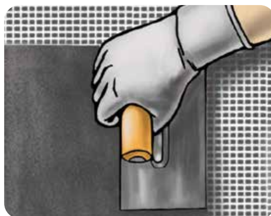
• Apply a second coat of MAGIFLEX after 4-8 hours, depending on the room temperature.
