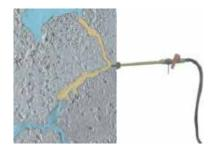
The liquid monomer solution activated in the aqueous phase begins to flow thanks to the high fluidity and Newtonian flow behaviour. **DRACOGEL GT2** continues
