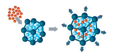
The polymerisation will be reactivated and the ingress water will be absorbed. DRACOGEL GT2 can swell to up to 30% of its volume, thus sealing cracks and recreating containment pressure to ensure waterproofing.
