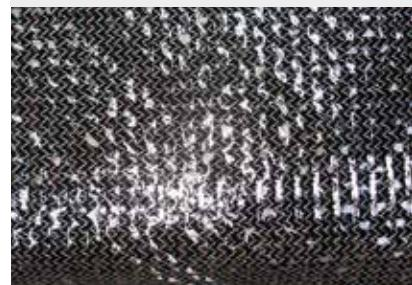
TKANINE I LAMELE OD UGLJIKOVIH VLAKANA ZA UČVRŠĆIVANJE I KONSTRUKCIJSKU ARMATURU
