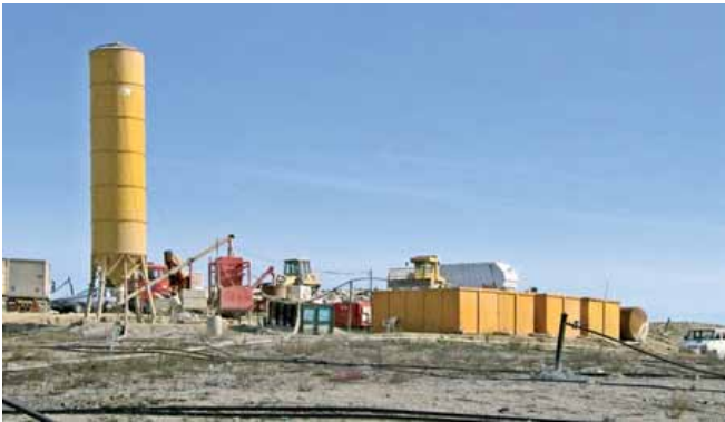
The use of the DRACRIL B.C. admixture eliminates the need for bentonite pre-activation tanks.
