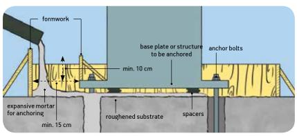
To guarantee a durable anchor point it is necessary to prepare the substrate properly, inspect the anchor cavities and check the conditions of the machinery before making the formwork
